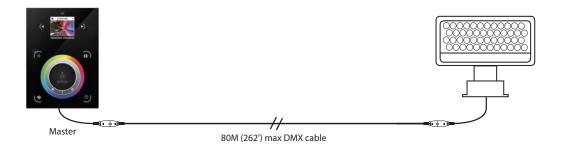
**NOTE**: More than 80M (252FT) of DMX cable requires an amplifier. More than 60 fixtures requires an amplifier.
