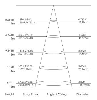
**Note:** The curves indicate the illuminated area and the average illumination when the luminaire is at a different distance.
